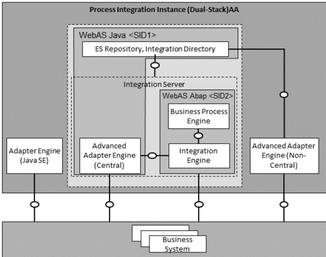
Figure 4: System Landscape for Building Integration Scenarios with PI Standard Installation
